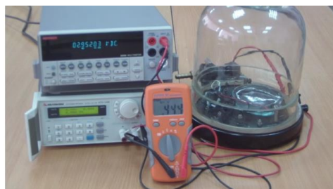
Figure 2 . Stand for measuring the output signal of the humidity sensor
