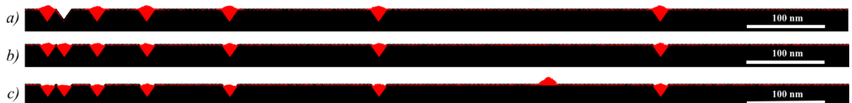
Fig. 3. Simulated morphology of droplet arrays obtained on patterned surfaces at different temperatures: a) 250°C, b) 200°C, c) 150°C.
