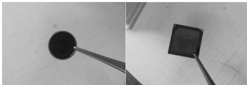
Fig. 1. a - Appearance of the finished silicon wafer, b - Appearance of the wafer for control before chemical rounding.
