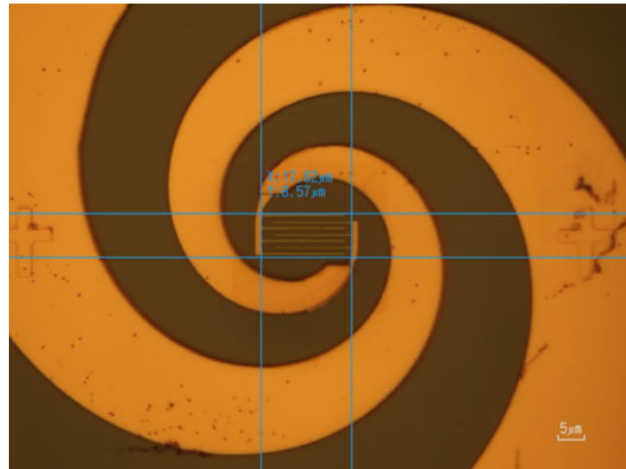
Figure 1. THz photodetector based on graphene, designed with an antenna for coupling the sensing element with radiation.
