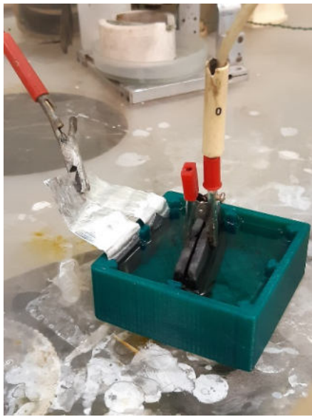
Figure 1. Electrochemical cell for the production of porous silicon and the result of simulation an electric field in Comsol Multiphysics
