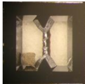
Figure 2. Degradation of the original cell topology after deep silicon etching during 6 hours in 30% KOH
